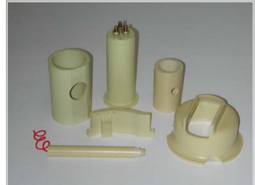
Selection of high density x-ray shields. Top right, typical shield for a dental tube application. The 1/4-inch shield wall thickness is equivalent to 1MM of lead lining. The shield both supports the x-ray tube insert and forms the beam at the port hole. Center, radiation shield with molded grooves for lead wires. Bottom left, shielded terminal support.
