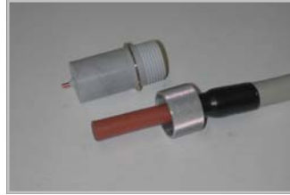
H190 mini plug (LGH-4) molded from EPR for vulcanized termination to cable insulation. Rated to 60KV, 1-2 conductors (H234 receptacle).
