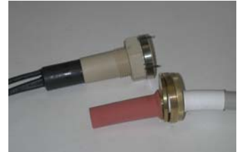
H435 mini plug with recessed pins molded from EPR for vulcanized termination to cable insulation. Rated to 75KV, 1-4 conductors (H1010 P2 receptacle).
