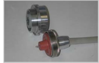
H189 compact plug molded from EPR for vulcanized termination to cable insulation. Rated to 60KV, 1-5 conductors (H78 receptacle).
