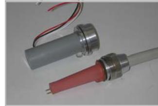
H199 keyed taper plug molded from EPR for vulcanized termination to cable insulation. Rated for 75KV, 1-4 conductors (H138 receptacle).
