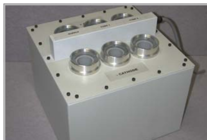
H850 P1 switch tank for two tubes, 220 VAC, 50/60HZ. High dielectric oil filled. 13"L x 13"W x 9"H. 45 LBS.
