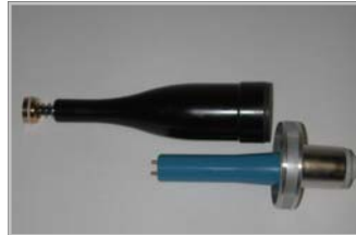
ML style bi-plug shown with "coke bottle" adapter used in Seifert and Philips tube towers. PMI integral "coke bottle" termination (photo below) eliminates bi-plug/adapter combination which frequently results in premature burnout of contacts due to electrical instability and overheating.
