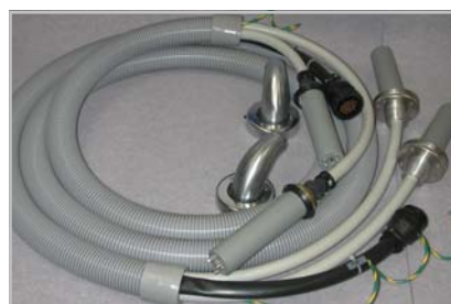
C-arm harness in flexible "old-style" hose with federal standard terminations.
