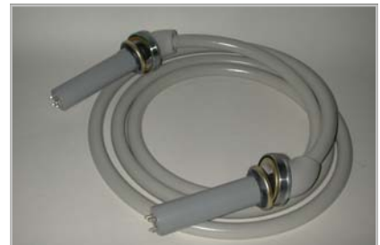
GE AMX cable assembly with 3-pin wide-flange federal terminals with fixed molded 45-deg strain reliefs.
